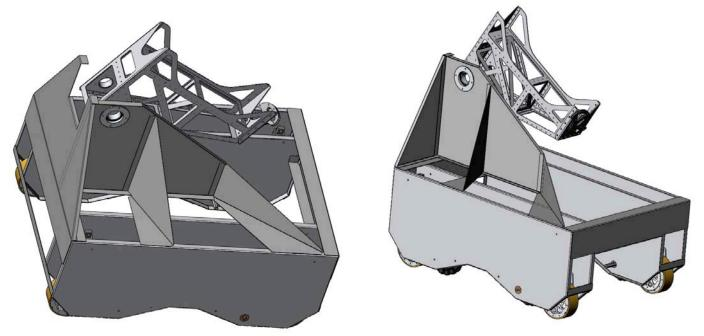
The 217-prototyping kids were working on the hanging mechanism; building a proof of concept mockup. They learned that the hanging claw design did not exert enough force on the bar to hold the robot in place. They ran the calculations and determined that shortening the claw would result in the robot holding; a revised mockup verified their calculations.
