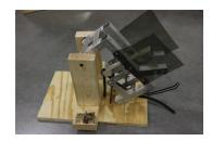
**Initial Prototypes:** When we began prototyping our shooter for this season. we quickly came up with multiple unique designs mainly made out of wood and other materials laying around out shop. These included a "flicker" design that quickly popped the balls forward, and multiple flywheel shooters, in various orientations and styles.
