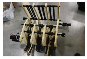
**Simplicity Is Key:** Soon after we made these initial prototypes, we quickly realized that ball collision in the air could severely hinder shot accuracy. This was dependent on the exit angle, orientation, and velocity. As such, we made the decision that we would settle for a single stream shooter, with the ability to shoot as fast as the robot would allow.
